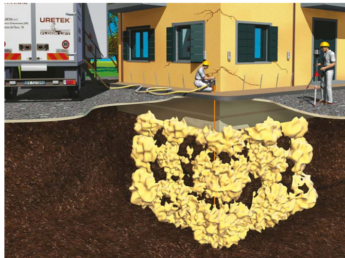
Figura 62. Uretek Deep Injections®.
