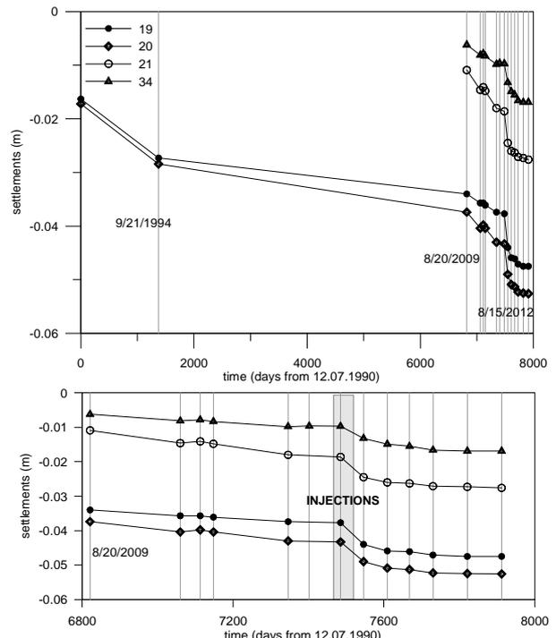
Figure 14. Above: Time-settlement curves of several anchorages. Below: enlargement of the measurements just before and after intervention
