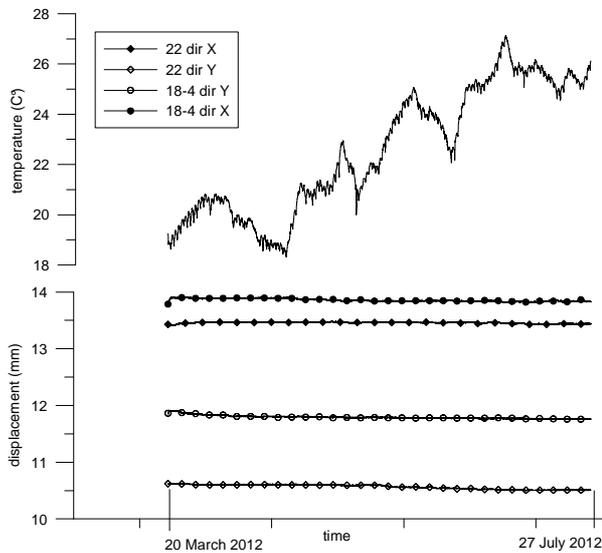
Figure 16. Time- displacement-temperature curves for two cracks (in X and Y directions)
