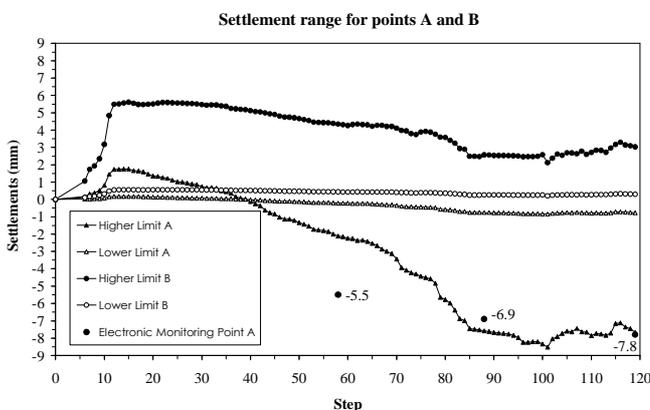
Figure 6. Time-settlement calculated curves and real measurements at Città di Castello tower
