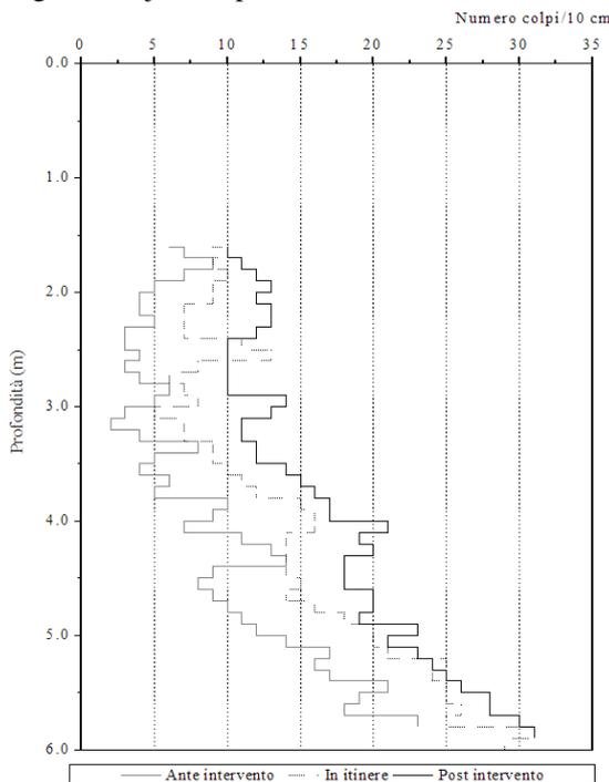
Figure 4. Penetrometer tests before and after intervention at Palatium Vetus
