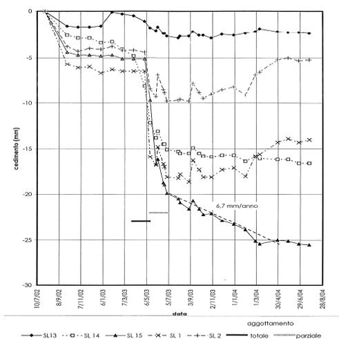
Figure 8. Time-settlement curves of several anchorages
