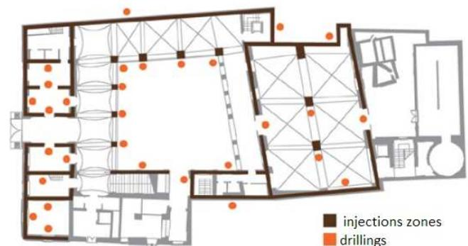
Figure 2. Above: foundation survey at Palatium Vetus. Below: survey and intervention map
